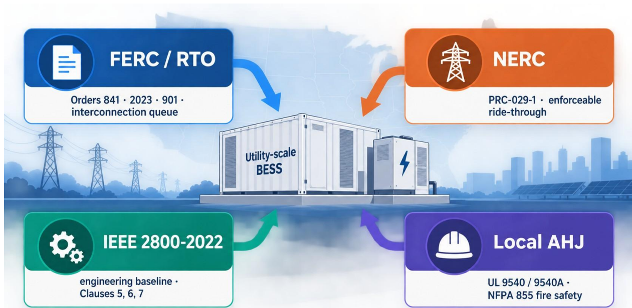
Figure 4. The four authorities a US battery project must satisfy.
